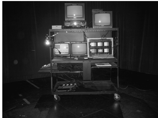
Figure 11.1 This cart on wheels has a switcher, an audio board, a graphic generator, and monitors for each camera, preview, line, and return feed.
