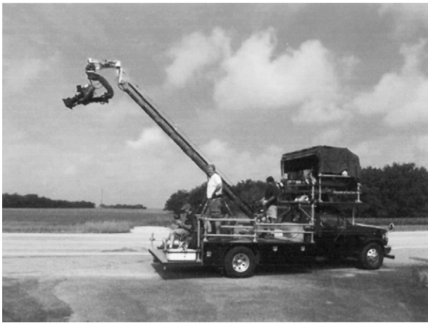
Figure 11.7 A Chapman Gryo-camera car Super VI on the road. This was configured with a vibration isolator and a gyro stabilized head. As configured, it's the kind of mount that's most often used in film or single-camera productions. Photo courtesy of Chapman/Leonard Studio Equipment, Inc.
